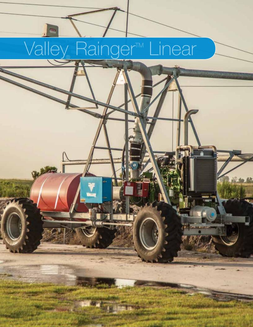
The Valley Rainger provides water source versatility with Ditch (canal) and Hose (pressured pipeline) Feed, and also has customized cart options. Valley Rainger™ Linears offer high flow capabilities that are not available with other mechanized irrigation equipment.
